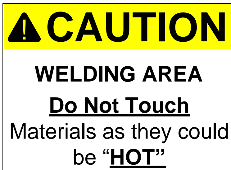
Figure 2, to be posted whenever hot work is left unattended
