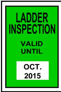
The green inspection label shown at left is placed on a fixed ladder that meets or exceeds the requirements of OSHA 29 CFR 1910.27, Fixed Ladders, and/or ANSI A14.3, American National Standard for Ladders – Fixed – Safety Requirements whichever was applicable at the time of installation.
